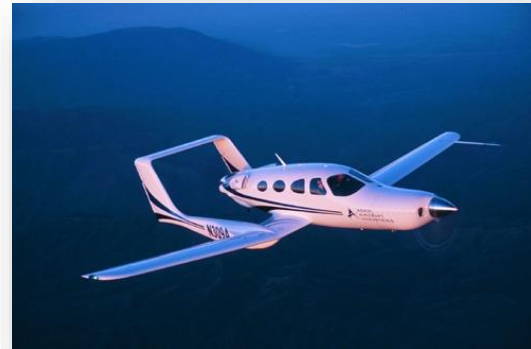
M-309 civil utility aircraft demonstrator has an airframe largely built of carbon fibre composite materials
