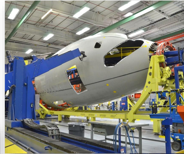
Boeing 787's Section 41 The first composite fuselage section for the first composite commercial jet | CompositesWorld
