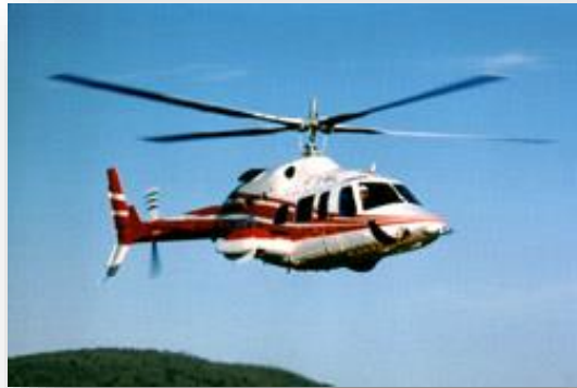
Helicopter Bell 430 uses composite systems in the blades and the fork that holds them
